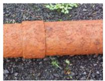
Photo 1. Iron on Well 2 Column Pipe, 2017.
