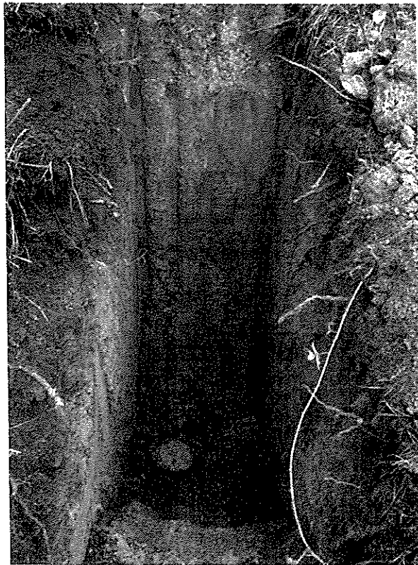
Photo 18 – View of the variable clayey silt and clayey sand exposed in Test Pit-11.
