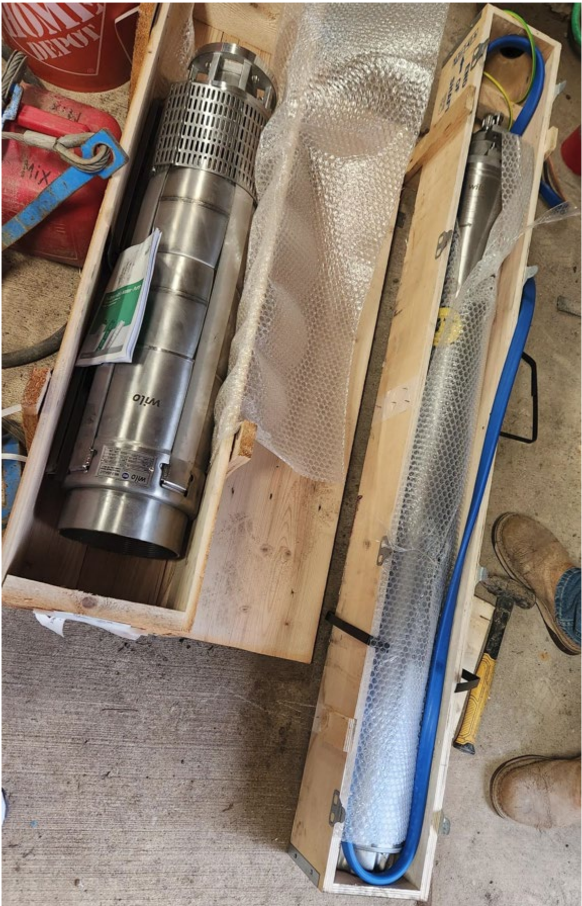
Down hole pump and motor for Well #3
